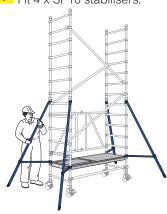
8 Fit 4 x horizontal braces (red) as quardrails 3T method, on the 11th and 13th rungs.
