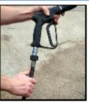
Attach trigger to high pressure hose.
