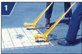
Use the EZI-LIFT inverted to break the seal of tight covers
