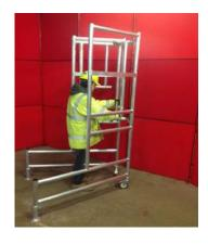
2) OPEN FRAME AND LOCK MECHANISM
