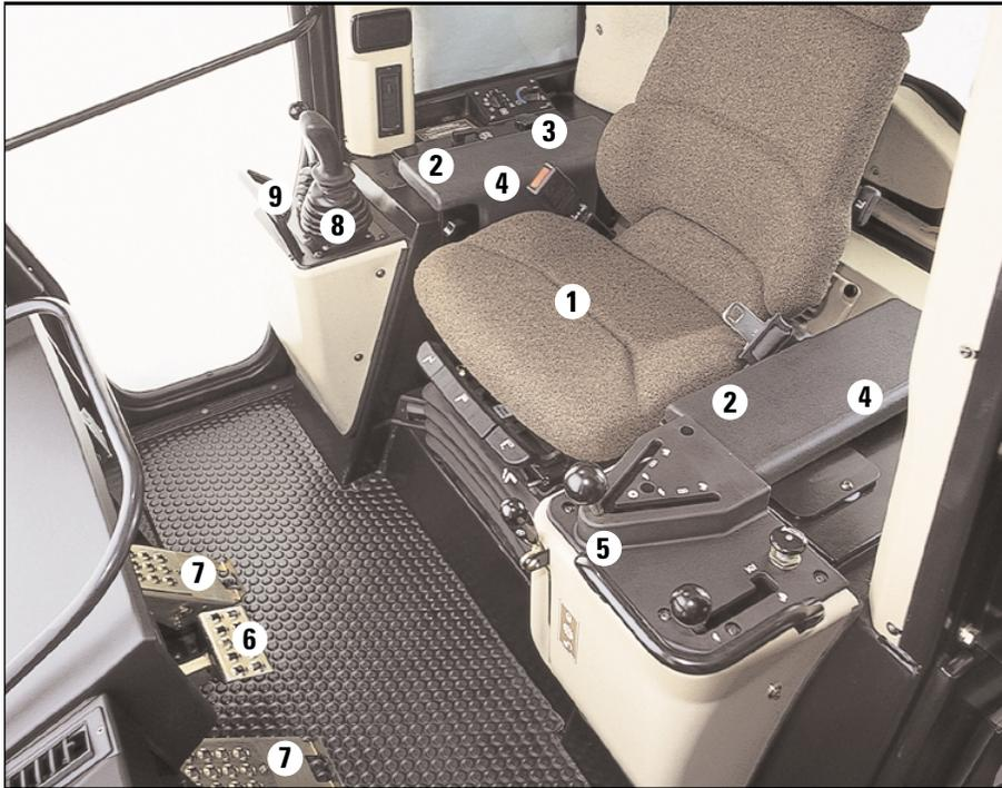
**1 Caterpillar Contour Series seat** is ergonomically designed and fully adjustable for maximum operator comfort and control — throughout the work day.
