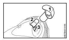
The spark plug boot (2) is under the cap (1).
