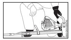
Put the unit on the ground: It must rest securely on the engine flange and the support on the frame.
