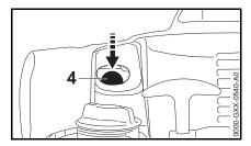
Depress the manual fuel pump bulb (4) at least five times – even if the bulb is filled with fuel.
