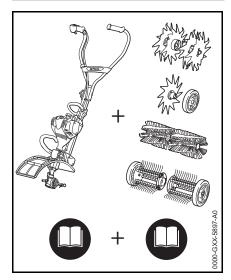
In the STIHL MultiSystem a number of different MultiEngines and MultiTools can be combined to produce a power tool. In this instruction manual the functional unit formed by the MultiEngine and MultiTool is referred to as the power tool.
