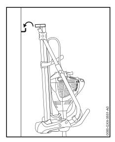
Fold the handle down and hang up the machine by the handle support.
