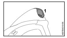
Push the cap (1) on to the spark plug boot as far as stop.
