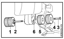
Push the extra weight (1) with bolt through the bore (6) in the flange, turning it until the square end (2) engages the recess in the flange.
