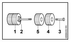
The weights (1) on the side with the square end (2) remain on the bolt.
