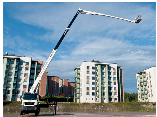
Fig. 2. S 50 XDTJ offers 16 meters up-and-over reach.
