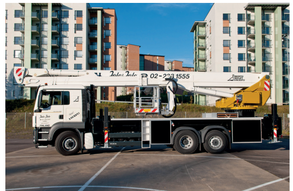
Fig. 1. S 50 XDTJ mounted on MAN TGS 26.400 6x4 chassis.
