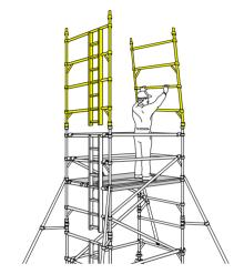
Fit 2 more diagonals between the 5<sup>th</sup> and 7<sup>th</sup> rungs. Fit a trapdoor deck on the 8<sup>th</sup> rungs of the tower. Fit a fixed deck next to it.
