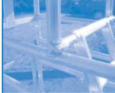
9. Remove the clip on tread from folding frame and replace them with the booster ladder ensuring that the clip on hooks are engaged around the frame uprights. Check that the unit is level, any brakes are on. Before starting work close the gate behind you using the drop down latch.
