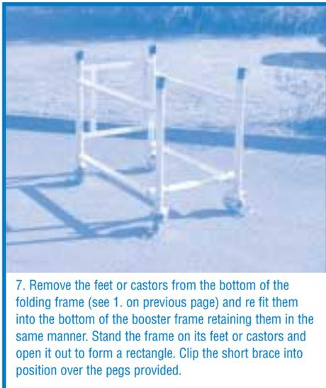
7. Remove the feet or castors from the bottom of the folding frame (see 1. on previous page) and re fit them into the bottom of the booster frame retaining them in the same manner. Stand the frame on its feet or castors and open it out to form a rectangle. Clip the short brace into position over the pegs provided.
