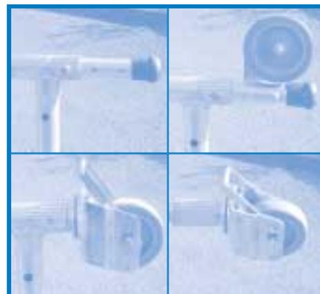
1. If not already installed, fit appropriate base option into the bottom of the folding frame. Feet and offset wheels are retained by nut and bolt, castors by friction lock and adjustable leg is secured by spring loaded pin.
