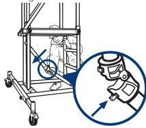
**IMPORTANT:** Do not let go of the platform and let it drop down under its own weight as this could cause damage to the work station. Hold onto the unit where labelled LIFT HERE and lower it with care.
