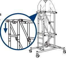
5 **IMPORTANT:** Facing the platform, climb down the ladder section. Never work when standing on the ladder section of the work station.
