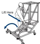
4 IMPORTANT: Ensure the diagonal strut locks into position, and the release trigger of the locking joint is fully engaged.
