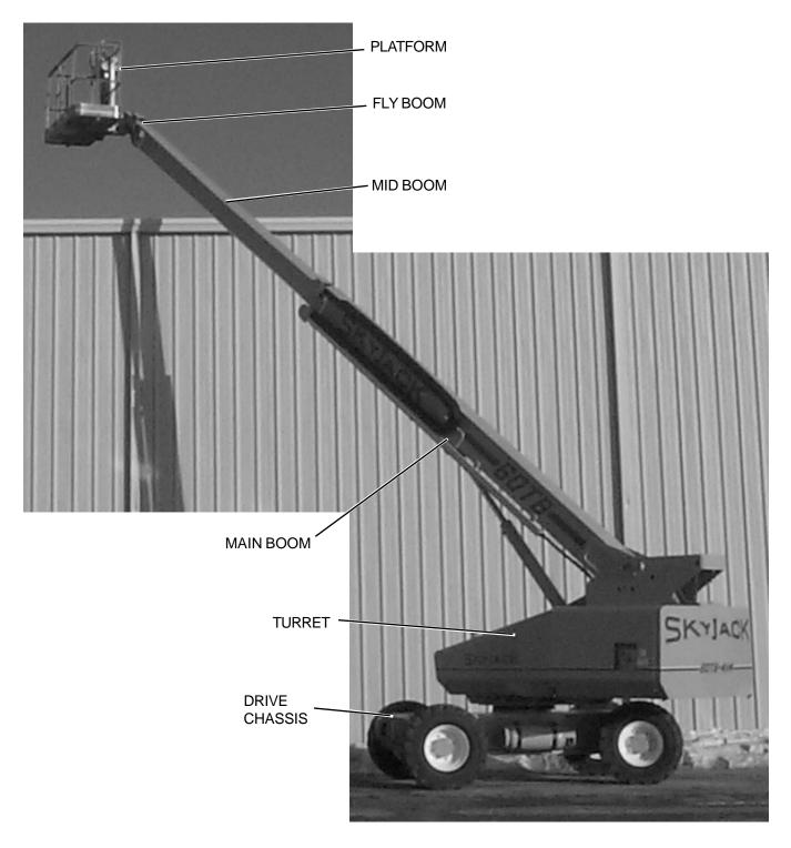
Figure 1-2. SKYJACK SJB Telescopic Boom Work Platform
