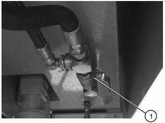
Figure 2-4. Hydraulic Fluid Shut-Off Valve
