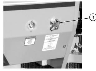
Figure 2-2. Battery Disconnect Switch
