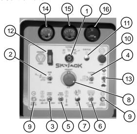
Figure 2-1. Base Control Panel and Label
