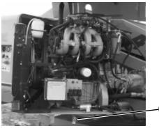
Figure 2-6a. Swing-out Engine Tray
