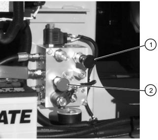
Figure 2-8. Brake Manifold
