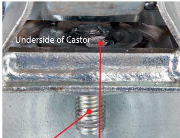
Underside of Castor Castor mounting bolt Swivel bearing head should feel free to rotate and not loose
