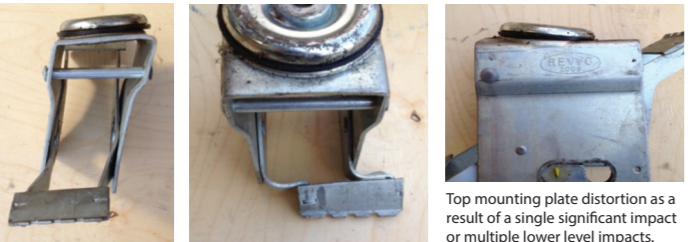
Side impact and foot pedal distortion as a result of a significant side impact. Foot pedal distortion as a result of a significant frontal impact; it is likely the top plate and bearing will be distorted as well. Top mounting plate distortion as a result of a single significant impact or multiple lower level impacts. Even if the rest of the castor is in good condition, it must be replaced.
