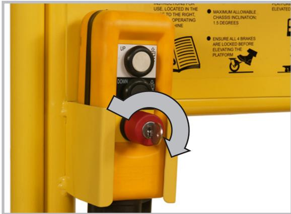
There is also an emergency stop button on the base unit. Push in to activate and twist clockwise to release.
