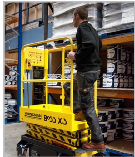
On entering the platform, ensure that the gate is closed behind you, as shown below.
