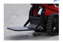
The Barreto 20HP Tracked Trencher, brought to you by The Hire Supply Company is the smallest dedicated tracked trencher on the market. Ideal for softer ground conditions the new tracked trencher has a larger ground contact area than conventional tyres. This gives lower ground pressure and greater traction. As well as being steerable so you can easily dig those corners and bends without having to reposition the machine.
