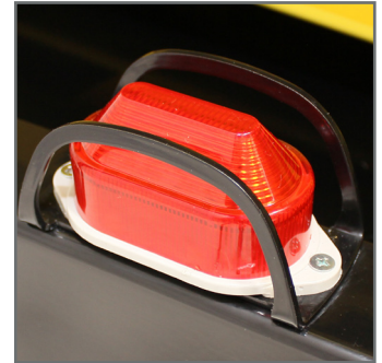
Warning lights and alarm on ascent/descent
