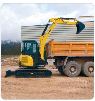
> For increased productivity the blade has been put forward by 20 cm. This allows better control of the job and better levelling. The blade lever, formerly cable operated, is hydraulic.
