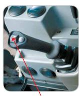
> The 3<sup>rd</sup> circuit of the hydraulic system is proportional in standard: easy use of accessories.
