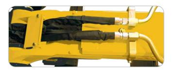
> Careful routing and protection of the hydraulic pipes on the boom and on the right side of the machine under the step. You can remove the step to access the sockets and change the equipment pipes.
