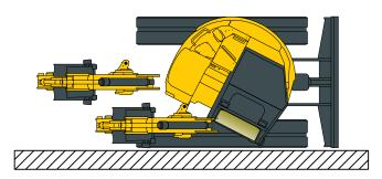
> Side ditch digging up to the wall with nothing sticking out beyond the track.
