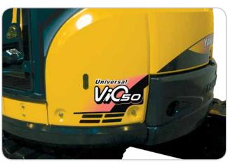
> Layout of the counterweight designed to protect the side panels against any possible shocks. Additional moulded parts at the left and right outer corners of the upper frame, improving shock resistance.
