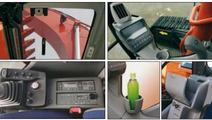
Wide adjustable armrests and a retractable seat belt are included. Short stroke levers allow for continuous operation with less fatigue. Three switches on the lever (optional) can be set to operate attachments other than buckets. The cab is pressurized to keep out dust. Noise and vibrations are kept to a minimum due to the elastic mounts, filled with silicone oil, the cab rests on.
