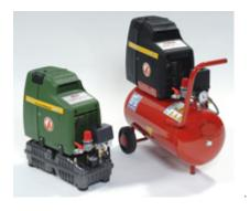
A range of receiver mounted, electrically operated oil free air compressors. All models are single phase (240V AC 13 amp). On/Off control is provided by an automatic pressure switch. Supplied with pressure regulator, gauge and shut-off valve.
