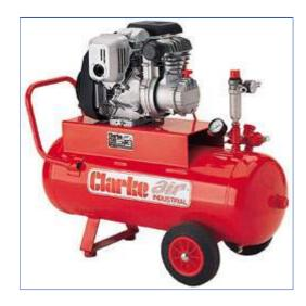
Powered by a reliable and rugged Honda petrol engine, this receiver mounted, engine driven air compressor is ideal for a wide range of outdoor, mobile applications remote from mains electricity.
