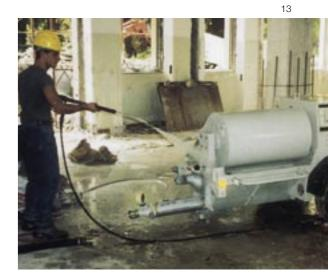
Pressure-clean your SP 11 using the built-in high-pressure cleaner and 140 bar water when the job has been completed (swivel discharge series).
