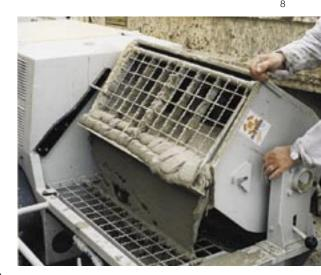
The swing mixer for the SP 11 DMB is comfortable to operate and makes light work of difficult jobs.
