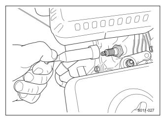
Remove the spark plug cable
