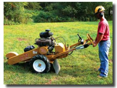
Handle bar is height adjustable and equipped with an operator presence safety shut-down bar.
