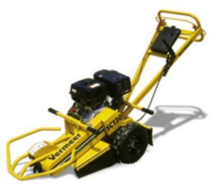
A cut above. The SC130 is portable and easy to maneuver, but its greatest attribute is the cutter wheel. Smooth cutting and long lasting, it takes only a few minutes to change using just 2 - 9/16" wrenches. Composed of 12 tungsten-carbide teeth common on larger commercial units, the wheel is segmented into four sections. If a section becomes damaged, it can be changed without replacing the entire wheel. The result fast, economical replacement or sharpening of worn or damaged wheel segments.
