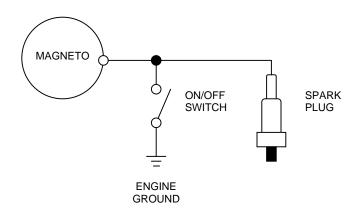
ON/OFF Switch Circuit Schematic Diagram Figure 5
