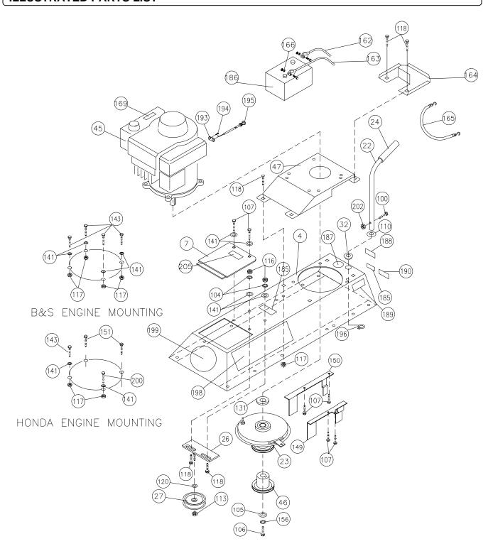
Engine and Engine Base Assembly Figure 6
