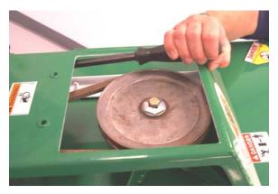
Adjusting Blade Drive Belt Tension
