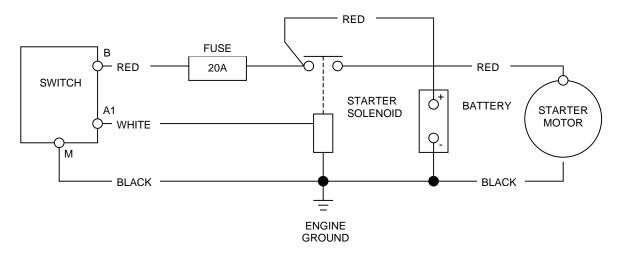
Starter Circuit Schematic Diagram Figure 4
