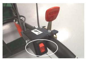
ON/OFF (I/O) Switch I-ON O-Off (Manual start shown)
