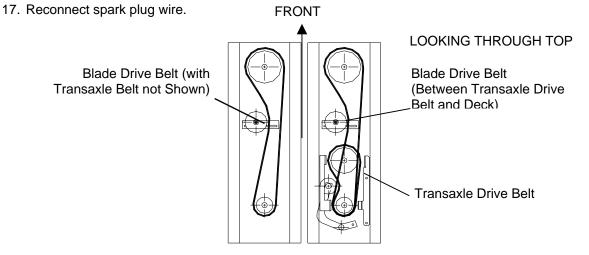
Belt Routing Diagram (Top View of Machine) Figure 2
