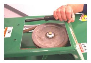
Adjusting Blade Drive Belt Tension
