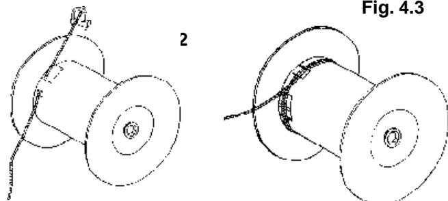
The rope must be attached in this way. Completely unwind the rope. Remove it from inside the drum through the hole and slot. Insert the new rope in the hole and thread it through the slot in the drum tube. Tighten the clamp at the end, leaving about 1 cm of rope free (fig. 4.2), and pull the rope until the clamp comes into contact with the inner wall of the drum.
