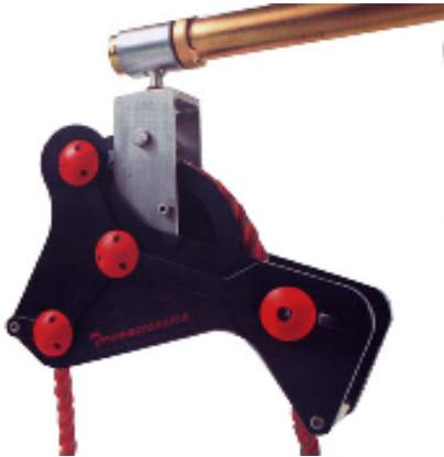
The exclusive automatic braking system locks the lifted load as soon as the rope is released by the operator.
