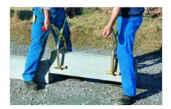
For the handling of kerb stones, edging stones, gutters & similar. Also can be used for natural kerb stones.
