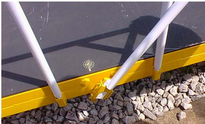
6. Check the brakes are working correctly – they are fail-safe so should be on when the Link Trolley is stationary.
