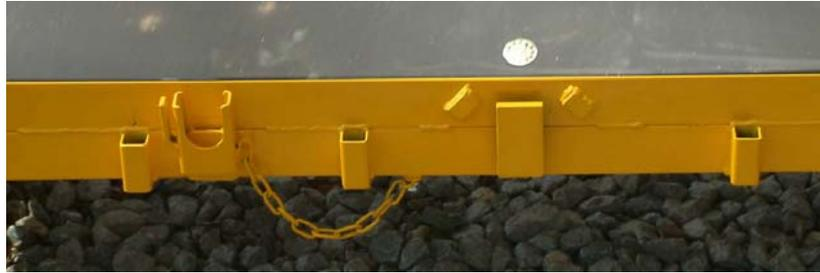
Move the Link Trolleys together so they are touching and connect the two together using the other Link Assembly, as shown below.
