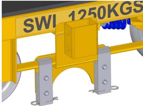
4. The flood light stand can be secured to the Light Bracket using the 2 holes in the aperture and suitable fasteners if required.
