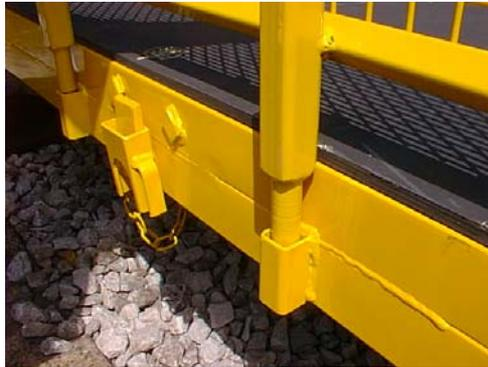
3. Slide the short Mesh Sides into the locating lugs, as shown below. Ensure that the top locking lug is engaged into the end frame of the long Mesh Sides.
