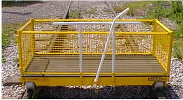
1. Mesh Sides (optional) are available to facilitate the loading of loose, lightweight and bulky items.
