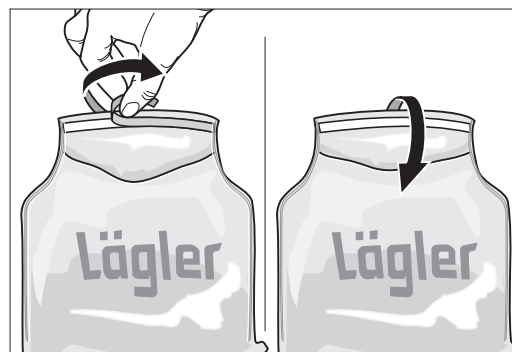
Fig. 15 Pull cover from the adhesive strip and seal the bag. The dust bag must be deposited in the open air!
