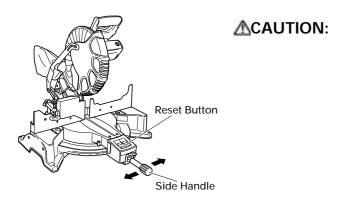
Move the turntable left and right with the side handle loosened and set it to the correct position.
