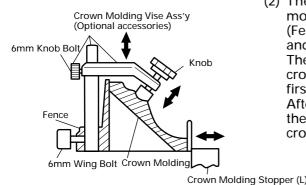
(2) The crown molding vise (B) (Optional accessory) can be mounted on either the left fence (Fence (B)) or the right fence (Fence (A)). It can unite with the slope of the crown molding and vice can be pressed down.
