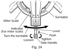
(1) Loosen the side handle and push the lever for angle stoppers. Then, adjust the turntable until the indicator aligns with desired setting on the miter scale (Fig. 24).
