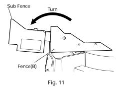
**⚠WARNING**: In the case of left bevel cutting, turn the sub fence counterclockwise. Unless it is turned counterclockwise, the main bady or saw blade may contact the sub fence, resulting in an injury.
