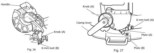
(1) Grip the handle on the motor head and position it at the bevel angle you need. Temporarily tighten the clamp lever.
