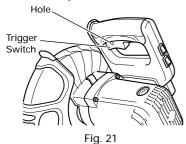
Pull the trigger to turn on the switch, release it to shut it off. After releasing the trigger, make sure the trigger has gone all the way back and the switch is turned off.
