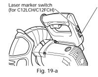
Digital display switch (for C12LCH/C12LC) (Also serves as laser marker power switch.)
