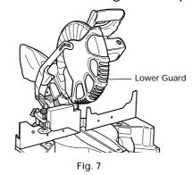
Lower guard is designed to protect the operator from coming into contact with the saw blade during operation of the tool. Always check that the lower guard moves smoothly and covers
