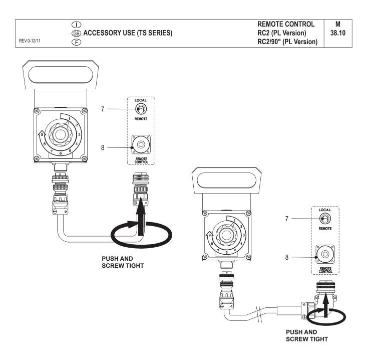
The remote control device for regulating the welding current is connected to the front panel by means of a multipole connector.
