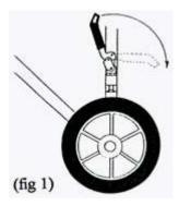
**B** Lock wheel brakes on (fig 1) then with man 1 standing on the hoop at the base of machine, man 2 raises the opposite end until machine bottoms on base hoop (fig 2).
