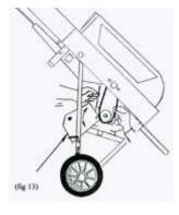
3. Rotate engine belt tensioner (fig 14) into place and operate lever to tension belts rotate belt, guard back up and lock fastener (fig 13).
