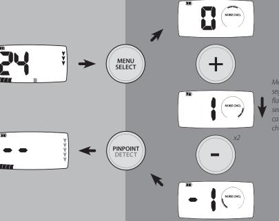
Menu scale segments will flash for 3 seconds while calibrating the channel
