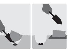
Check the hole for the target. If it is not in the hole, place the detector on the ground with the coil flat, pick up a handful of soil and pass it over the coil. Be sure not to wear rings, bracelets or a watch which will produce a signal. Repeat this procedure until the target is located.
