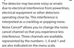
It is best to choose a channel with the coil in the detection (horizontal) position because interference received in a vertical position may be different from the interference received in the horizontal position.
