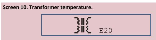
If the transformer inside the welding unit has become too hot the welding unit will stop displaying the screen above. Only when the transformer has returned to a working temperature will the screen clear.
