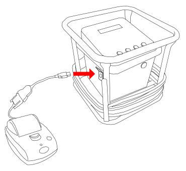
Switch the welding unit on, when the printer is detected the screen below is displayed.
