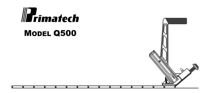
This manual nailer has been developed to work with 3/8" to 5/8" boards. It is a single hit nailer which drives  $1\frac{1}{4}$ " (32mm) and  $1\frac{1}{2}$ " (38mm) 18-GAGE L-type flooring cleats at the perfect location and angle. It comes with a set of plastic bases to precisely fit any solid boards.
