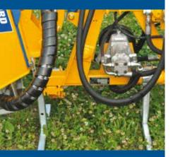
Fully independent hydraulics For continuous use. Twin pumps with separate oil tank.
