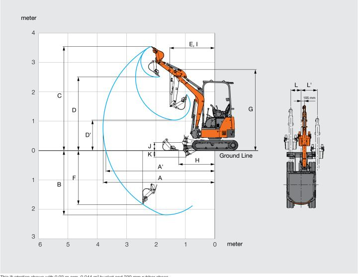
This illustration shows with 0.93 m arm, 0.044 m³ bucket and 230 mm rubber shoes.
