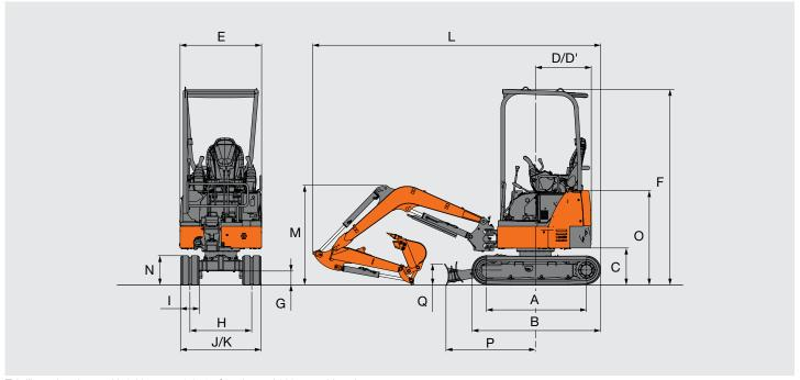
This illustration shows with 0.93 m arm, 0.044 m³ bucket and 230 mm rubber shoes.
