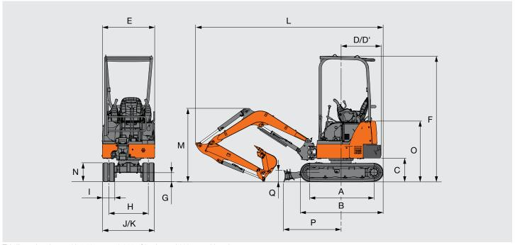
This illustration shows with 1.13 m arm, 0.044 m³ bucket and 230 mm rubber shoes.
