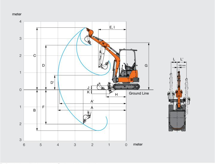
This illustration shows with 1.13 m arm, 0.044 m³ bucket and 230 mm rubber shoes.
